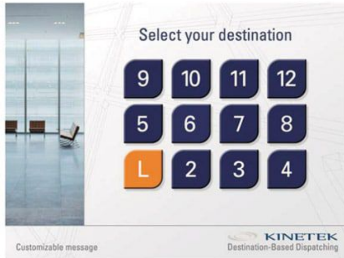
Passenger selects desired floor, then is directed to specific elevator.
